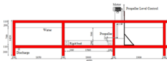
Figure 1 - Experimental set-up, Longitudinal cross-section (in mm).
