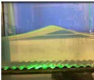
Figure 1 - PIV measurements of plastic debris velocity in the wave flume
