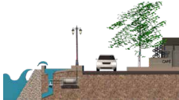
Figure 1 - Sketch of the Overtopping Device WEC Concept Located on a vertical sea wall
