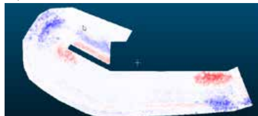
Figure 2 - Erosion-Accretion map of the breakwater
